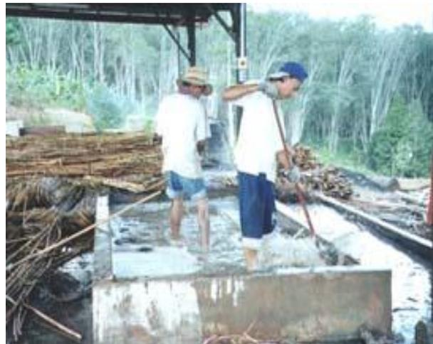
**Gambar 7. Proses pengawetan rotan (Sumber, Transfer of Technology Model, Rattan Furniture Making Unit, International Network for Bamboo and Rattan)**
